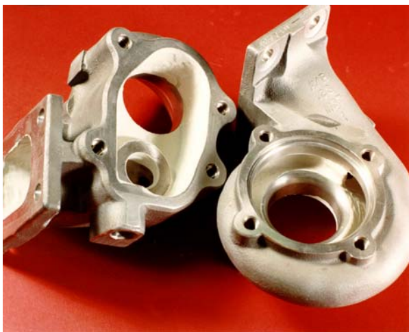
LT-450 Thermal Barrier Coating on Inside of Stainless Steel Turbocharger Scroll, Wastegate, and Throat Areas. Allows Coatings in Areas Where Other Coatings Cannot be Applied.
