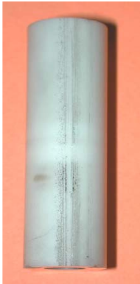
Al 2 O 3 Thread Guide Test Sample (after 80,000,000 feet)
