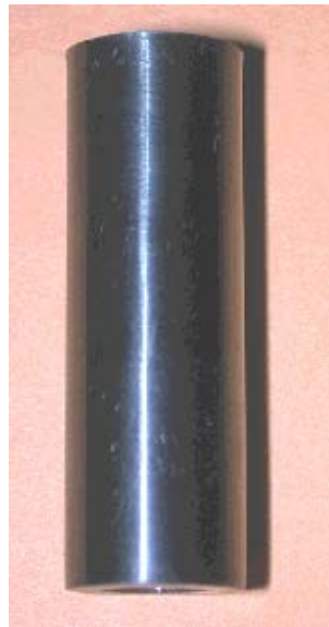
Thin Film Coated Steel Test Sample (after 80,000,000 feet)
